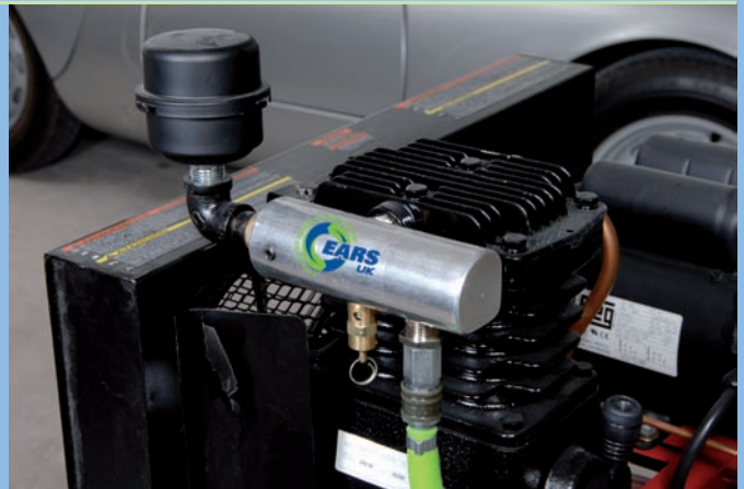
Installed E.A.R.S manifold
